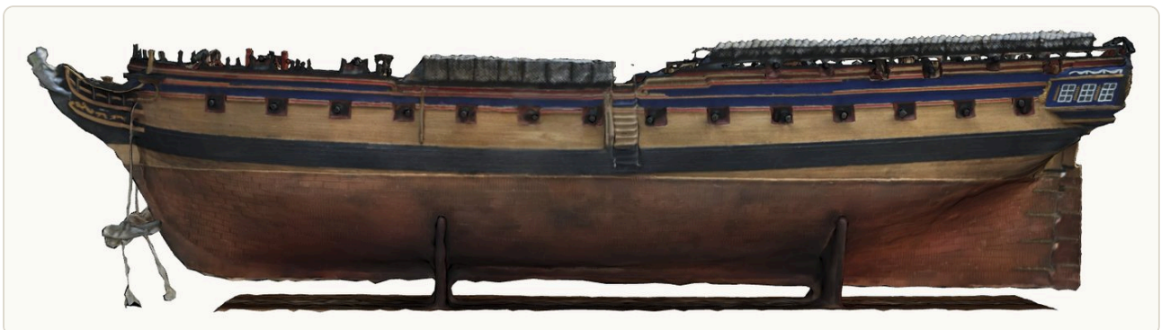
Attempt 2: outdoors in the shade, 1,103 photographs, with a separate pass round every fitting. Same ship, same phone.
