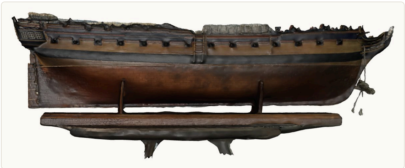
Attempt 1: indoors under lamps, 221 photographs from a metre away. The hull is blotchy, the bulwark is mush.
